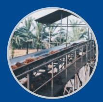
Palm Oil Mill scraper conveyor - Palm Oil is extracted from the bunches of fruits and the waste is conveyed away.
