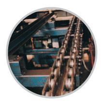
Special Double Strand Conveyor Chain used in a corrugated roofing plant in Chile.
