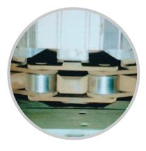
Conveyor Chain with Aluminium Slats for a continuous metal belt root crop conveyor.
