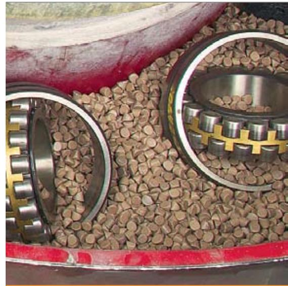
*Timken's bearing reclamation services can reduce your cost of operation by returning refurbished bearings to service.*
