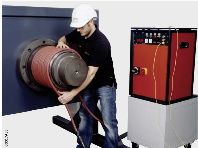
Figure 1 The flexible inductor can be wrapped around the component
