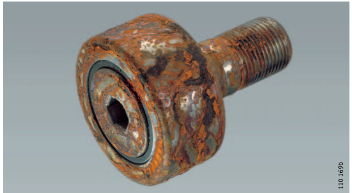
Figure 1 NUKR52 without coating after salt spray test
