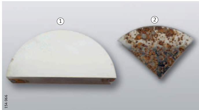
Figure 1 Corrosion resistance, comparison after 24 h in salt spray test
