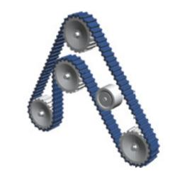
Figure 3.2.2: Multi-pulley drive with inside, smooth cylindrical pulley
